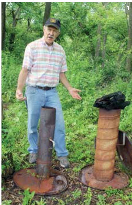
1. John Gibbs fashions these “chimney lids” that are placed on top of barrels in which the wood burns. The chimneys restrict the air in the barrels, enabling the wood to char instead of burn completely. 2. The charred pieces of wood are sifted through this machine, with smaller pieces dropping to the tray along the bottom. 3. The pieces packaged as lump charcoal resemble the wood it comes from. 4. Finer pieces create biochar, a soil amendment highly valued for its agriculture benefits.
